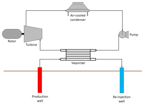
Figure 1: A diagram of a binary geothermal power generation system which utilises an air-cooled condenser for condensing the organic working fluid.
