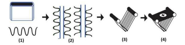
Figure 4: ACC assembly example. (1) Attachment of fins to tubes in a single row by brazing. (2) Tubes assembled into bundles. (3) Two bundles connected to the same header. (4) Fan mounting structure connected between the tubes.
