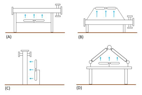
Figure 2: Different orientations of air-cooled condensers.
