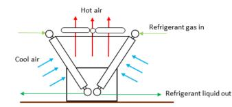
Figure 3: An air-cooled condenser in the "V" configuration.
