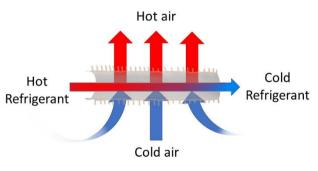
Figure 5: The general principle of the ACC.
