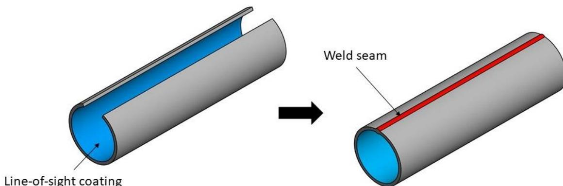
Figure 4: An alternative route of producing internally coated small diameter welded tubes coated with line-of-sight methods.
