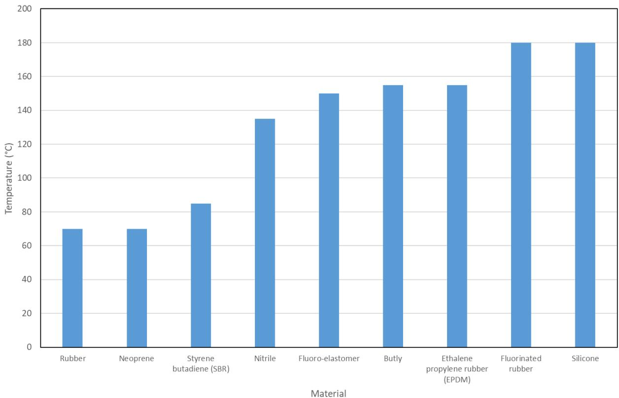
Figure 2: Maximum operating temperatures for various gasket materials.
