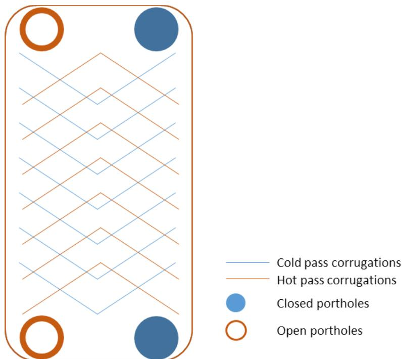
Figure 1: Schematic diagram of alternating chevron pattern orientations on successive plates of plate heat exchangers.
