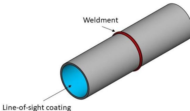
Figure 5: Another possibility of producing long small diameter pipes internally coated with line-of-sight methods.
