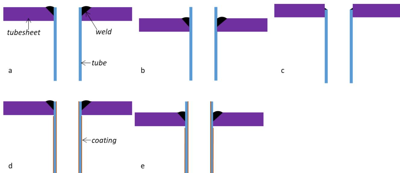
Figure 3: Weld configurations with a) Flush tube, b) protruding tube and c) recessed tube; Weld configurations for coated tubes: d) flush e) protruding.
