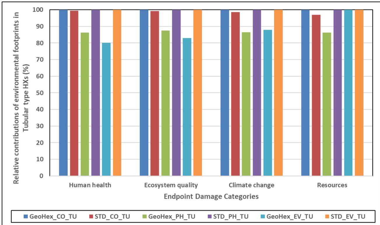
Figure 4.9 – Comparisons of environmental footprint contributions in 4 endpoint damage categories for 1 m<sup>2</sup> area of 6 tubular type HXs.
