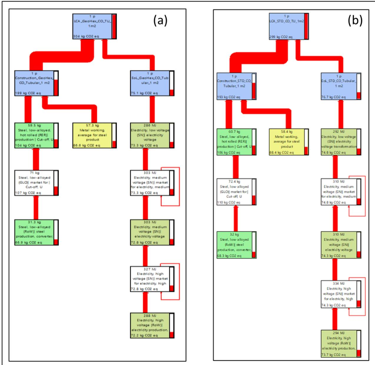
**Figure 4.7** – A part of the climate change network models for 1 m<sup>2</sup> area of (a) GeoHex enabled and (b) standard tubular type condensers.
