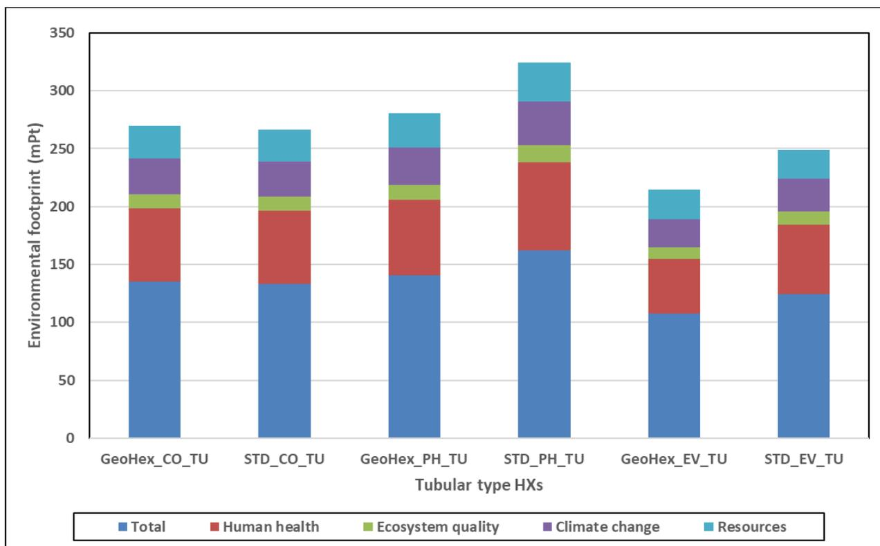
Figure 4.10– Total and four environmental footprint results in mPt for 6 tubular type HXs.
