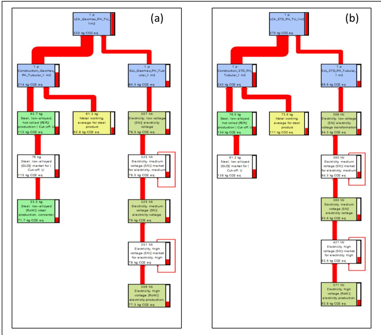
Figure 4.8 – A part of the climate change network models for 1 m² area of (a) GeoHex enabled and (b) standard tubular type preheaters.
