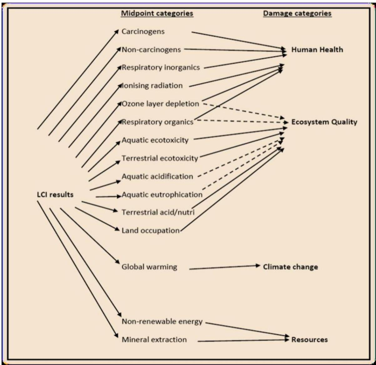
Figure 2.2 – Overall scheme of the IMPACT 2002+ framework.
