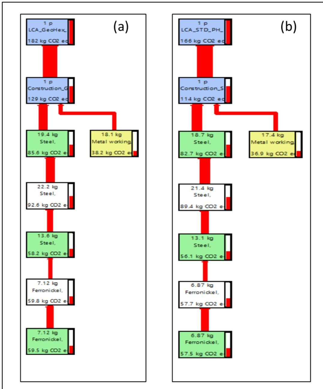
**Figure 4.3** – A part of the climate change network models for 1 m<sup>2</sup> area of (a) GeoHex enabled and (b) standard plate type preheaters.
