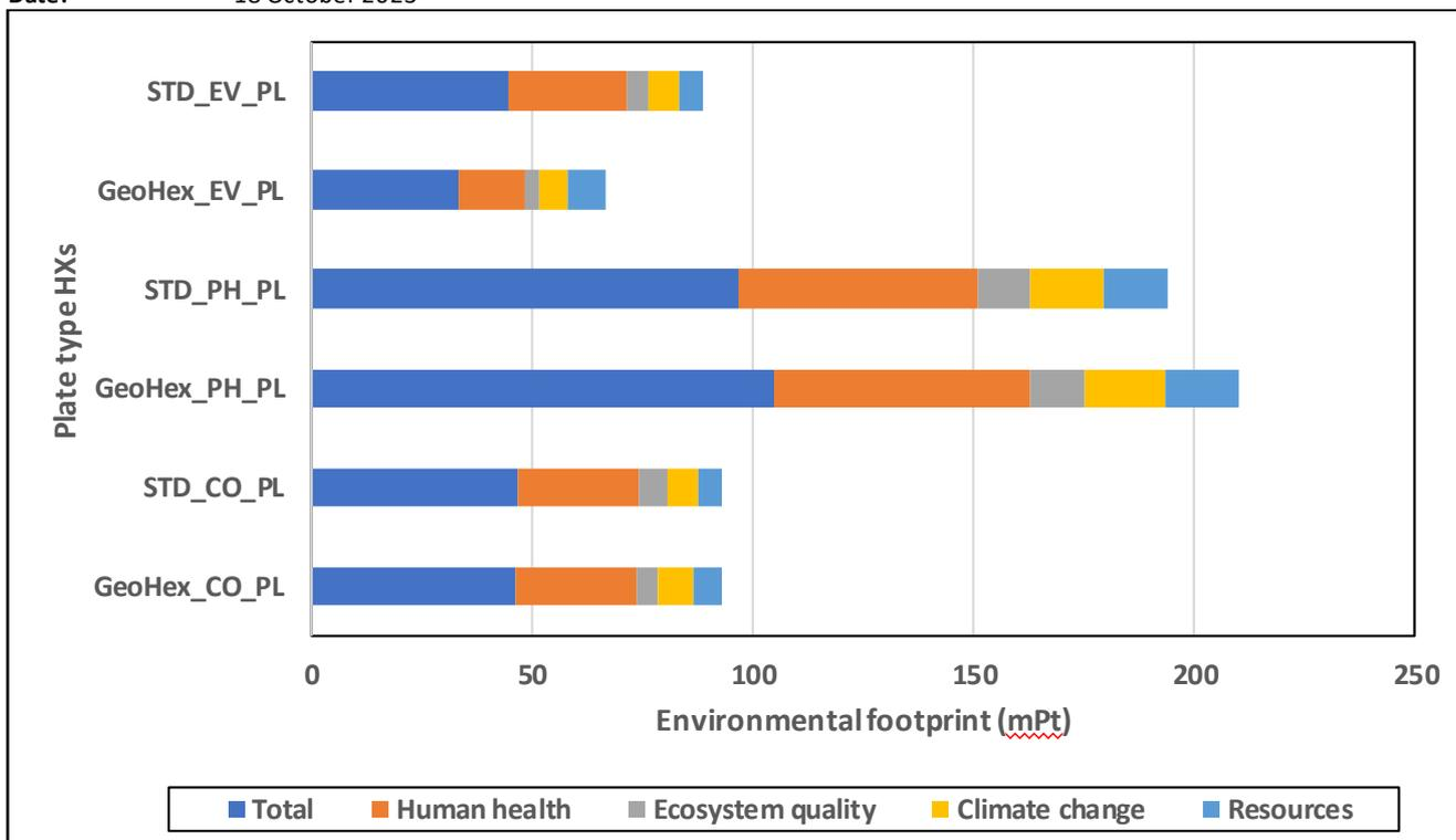
Figure 4.5 – Total and four environmental footprint results in mPt for 6 plate type HXs.
