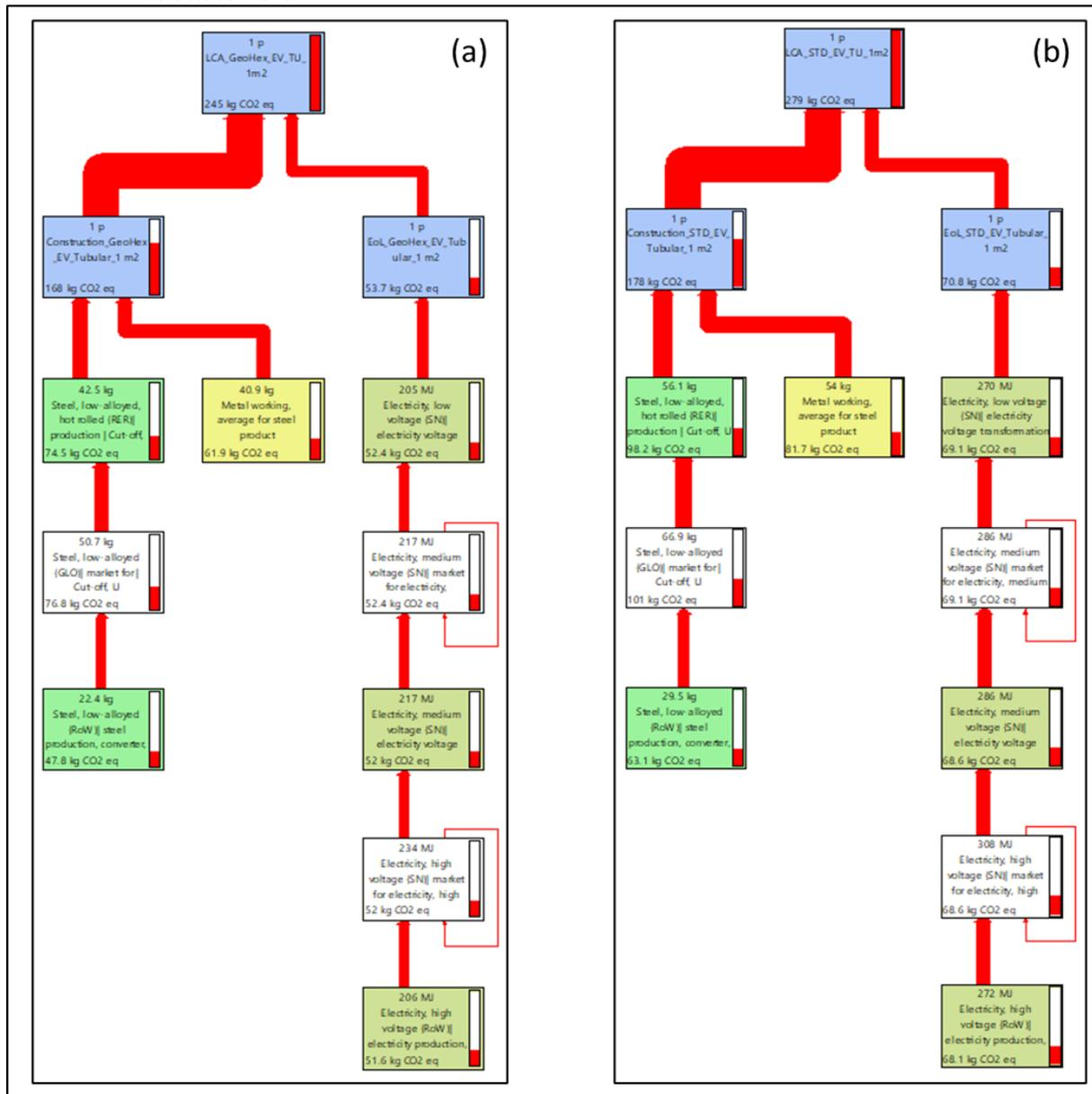
Figure 4.6 - A part of the climate change network models for 1 m<sup>2</sup> area of (a) GeoHex enabled and (b) standard tubular type evaporators.
