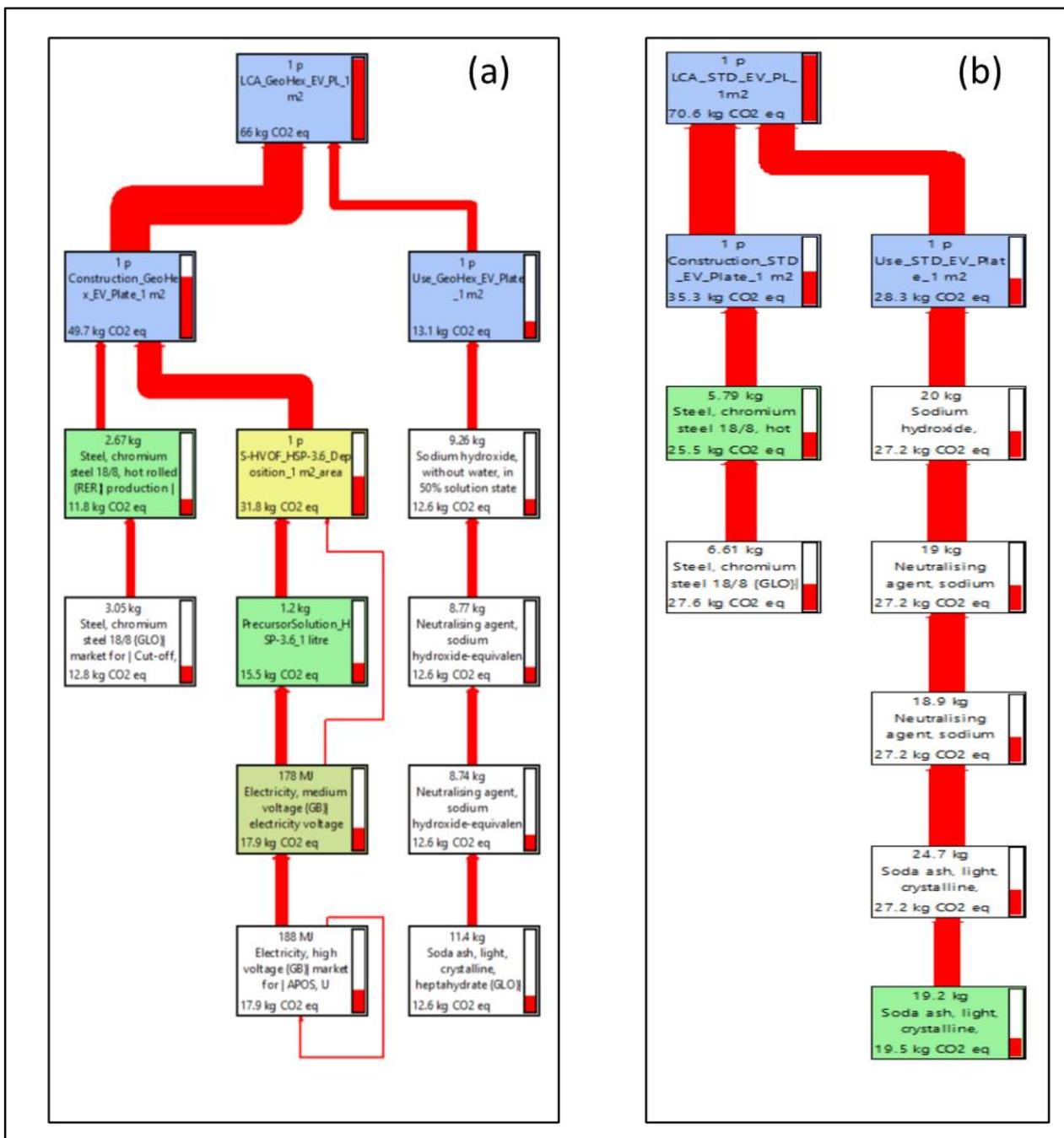
Figure 4.1 – A part of the climate change network models for 1 m<sup>2</sup> area of (a) GeoHex enabled and (b) standard plate type evaporators.
