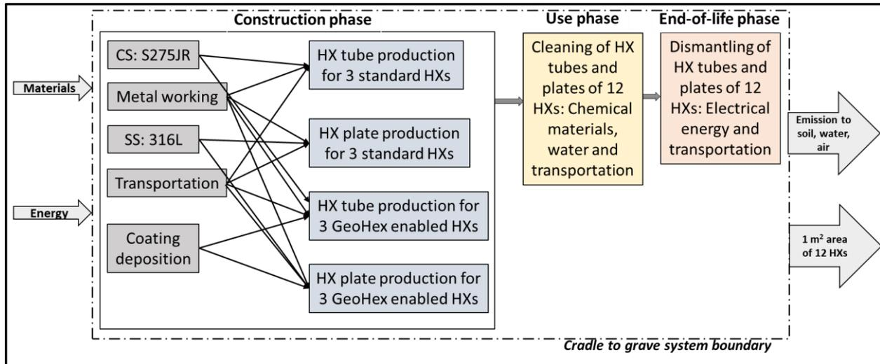
**Figure 1.1** – A cradle to grave system boundary of life cycle assessment (LCA) study of 12 HXs
