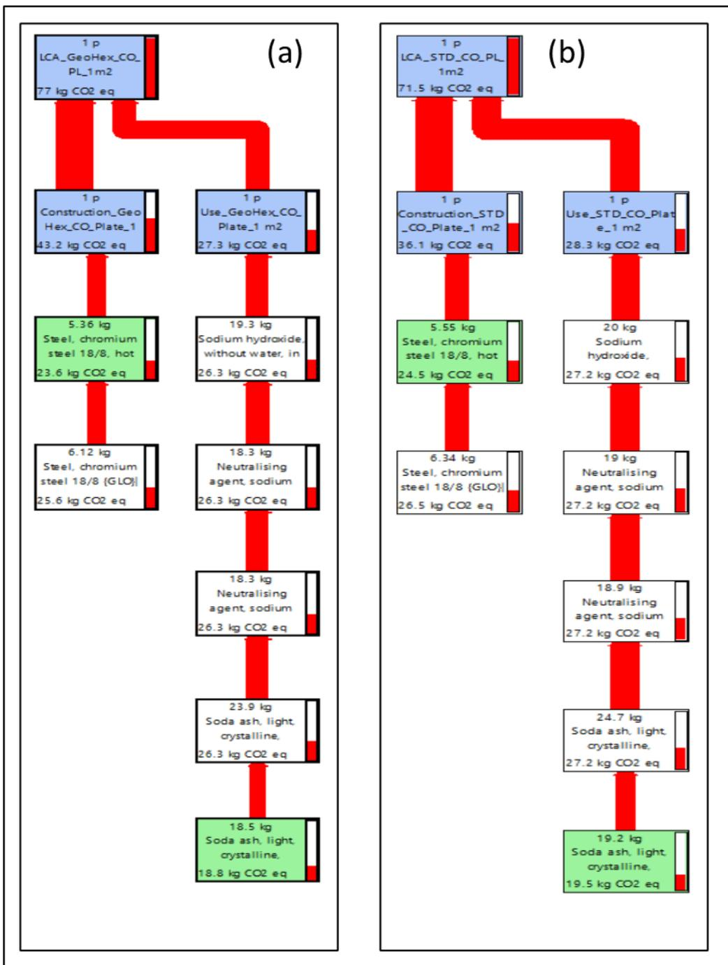
Figure 4.2 – A part of the climate change network models for 1 m<sup>2</sup> area of (a) GeoHex enabled and (b) standard plate type condensers.
