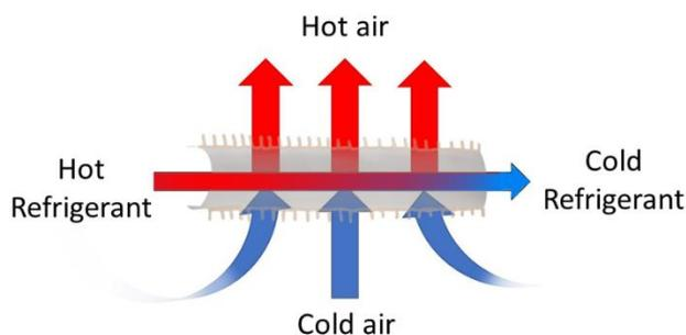
Figure 5: The general principle of the ACC.
