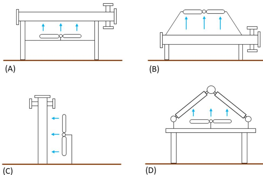
Figure 2: Different orientations of air-cooled condensers.
