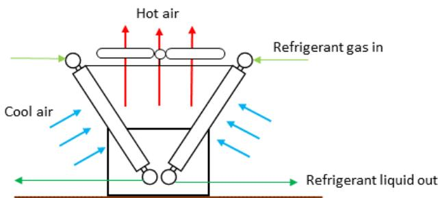
Figure 3: An air-cooled condenser in the “V” configuration.
