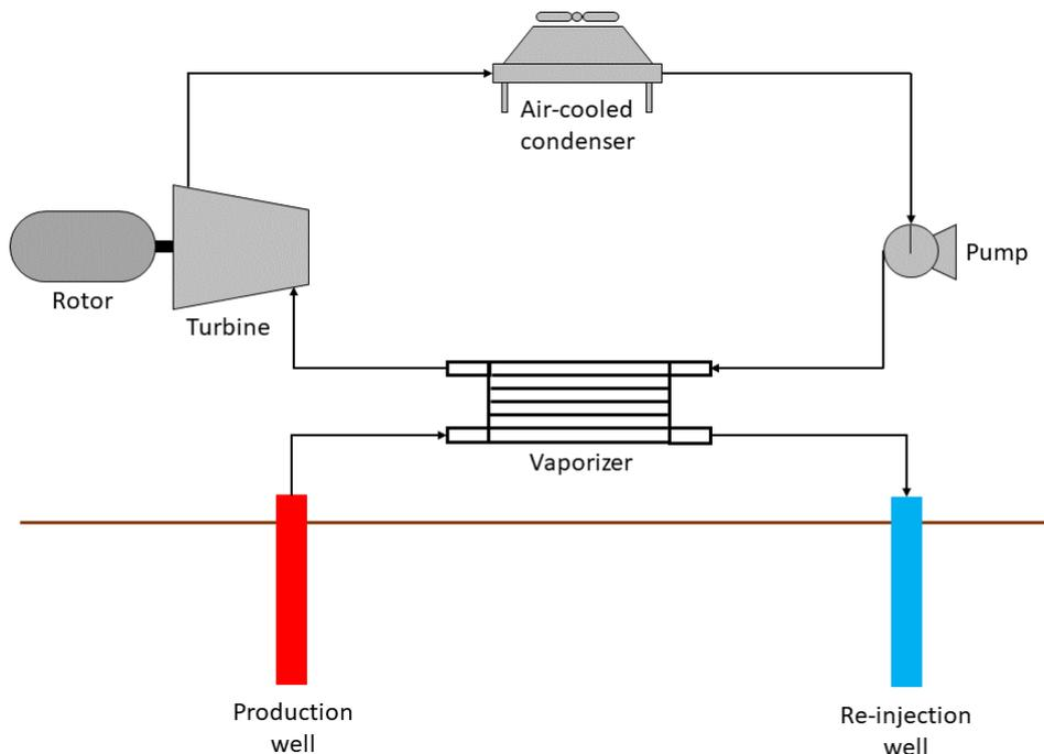
Figure 1: A diagram of a binary geothermal power generation system which utilises an air-cooled condenser for condensing the organic working fluid.
