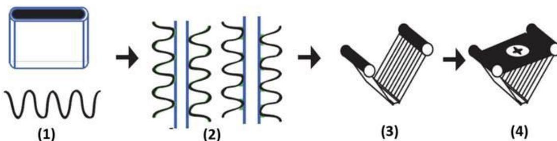
Figure 4: ACC assembly example. (1) Attachment of fins to tubes in a single row by brazing. (2) Tubes assembled into bundles. (3) Two bundles connected to the same header. (4) Fan mounting structure connected between the tubes.
